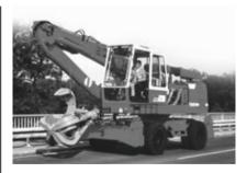
First hydraulic cab elevation
