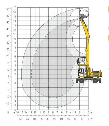
Height 👊 Can be slewed through 360° 🖟 In longitudinal position of undercarriage
