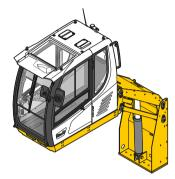
Hydraulic cab elevation
