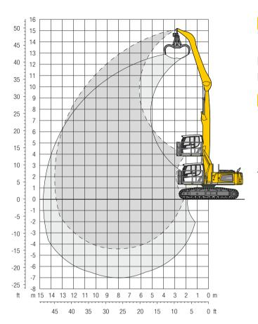
Height 🖰 Can be slewed through 360° 🖟 In longitudinal position of undercarriage
