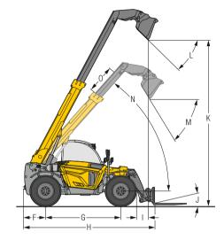
**Dimensions** (all specifactions with standard tyres, standard fork or standard bucket (0.9m³/1.18 yd³))
