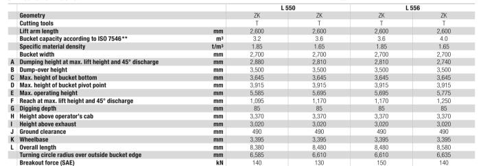
The figures shown include the above tyres, all lubricants, a full fuel tank, the ROPS/FOPS cab and the operator. Different tyres and optional equipment will change the operating weight and tipping load. (Tipping load, fully articulated according to ISO 14397-1)
